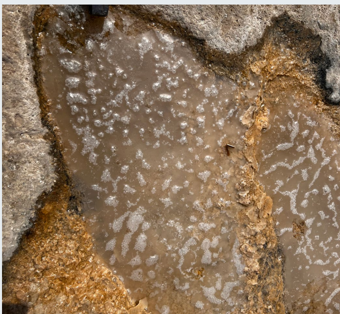
Figure 6: Calcium Carbonate crust trapping hydrogen bubbles
