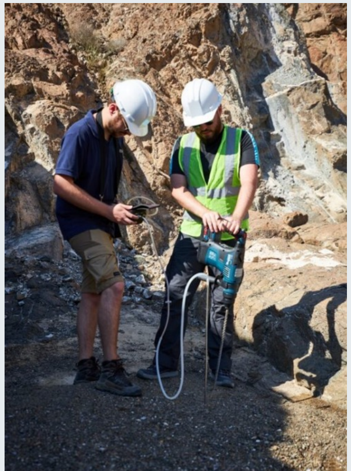
Figure 8: Measuring hydrogen anomalies in soil
