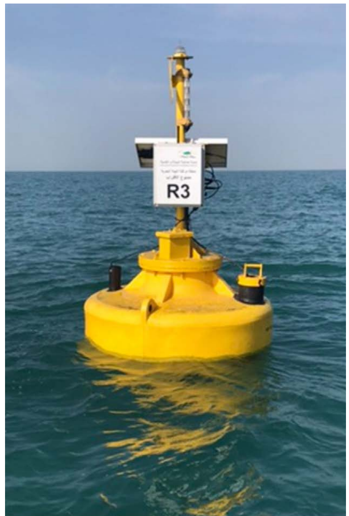
Figure 14: Floating water quality meter deployed to monitor marine conditions in Ras Al Khaimah
