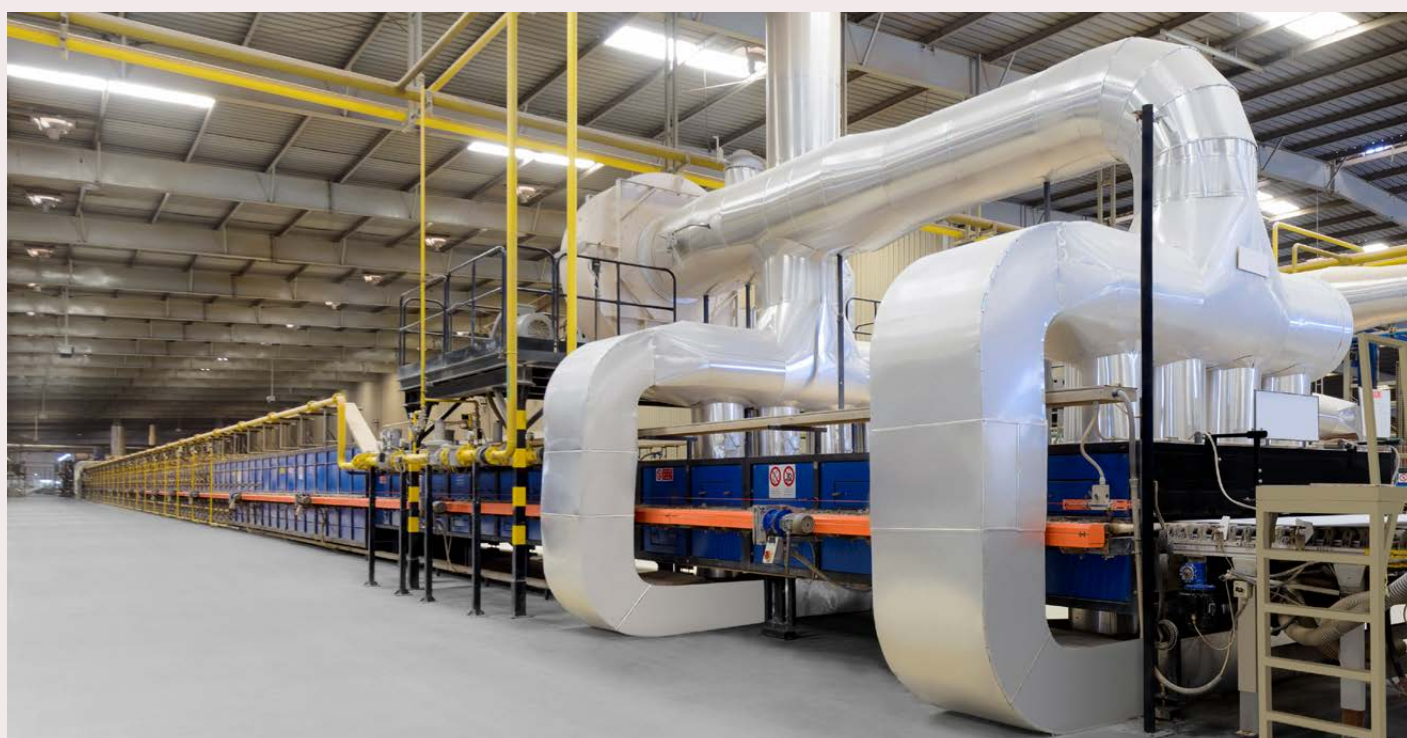
Figure 32: Waste heat recovery system at RAK Ceramics
